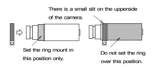
Fix the mount by passing the ring over the lens of the camera, and then attach the thread and nut.
