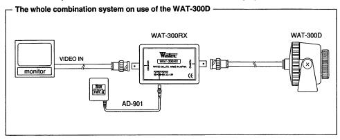
NOTE: A 3C2V or 5C2V coaxial cable with 75 $\Omega$  impedance must be used for connection between the WAT-300D and the WAT-300RX.
