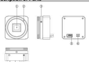
(1) IMAGE SENSOR FRONT FACE The light receiving face of the image sensor
